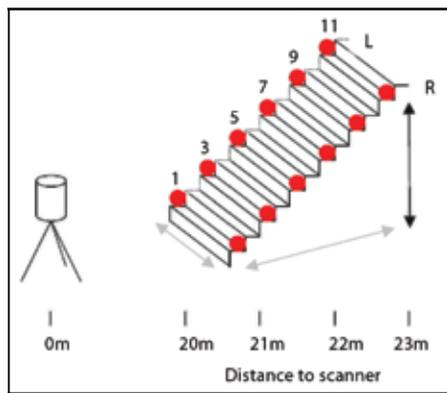
▲ Staircase test set-up used for determining important angular errors in scanners—
