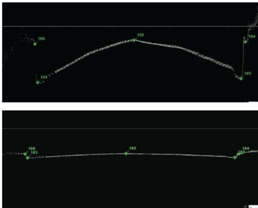
▲ Vertical exaggeration tool (see top image) in software helps users select best top-of-curb, bottom-of-curb, and high road surface points from scan data.
