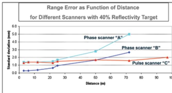
◀ Scanner range error increases with distance; errors increase at different rates for phase scanners and pulsed scanners —Image courtesy: i3Mainz
