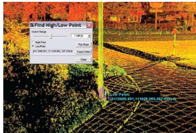
▲ Office software can automatically locate and select lowest and highest points from clusters of high-definition survey data.
