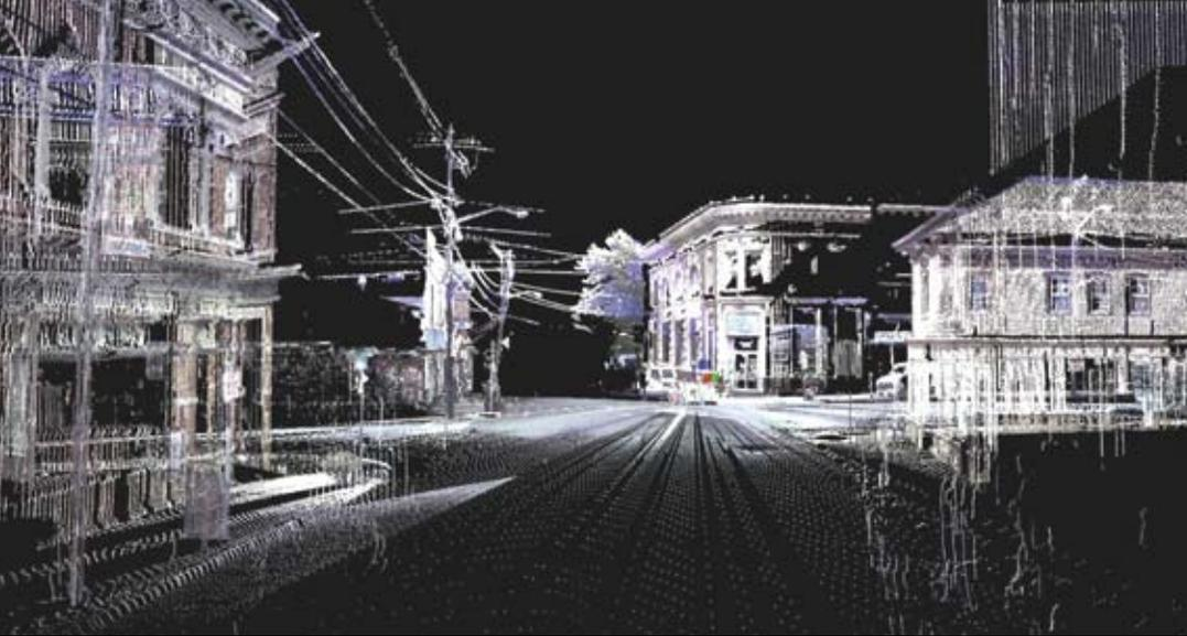
By capturing 3D building details, all overhead lines, and tree details, a high-definition survey can provide helpful context to supplement traditional 2D drawings for planning proposals—courtesy of MJ Engineering and Land Surveying.
