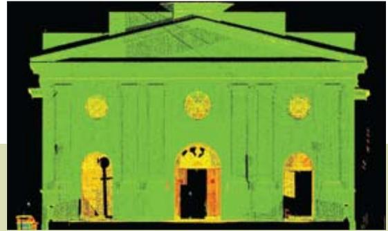
Special viewing modes in point cloud office software make it easier to interpret laser scan data for conversion into deliverables. Image on the right is in standard “intensity map” mode; image on the left is the same view, but using friendly “silhouette” mode.
