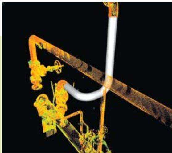
◀ Users can select a single scan point on a pipe to automatically create a piping run CAD object.
